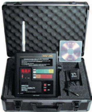
DSP2B/DSP2BP - DSP2B Dedicated Speech Intelligibility Meter Measures Sound Pressure Level and Speech Intelligibility Index
